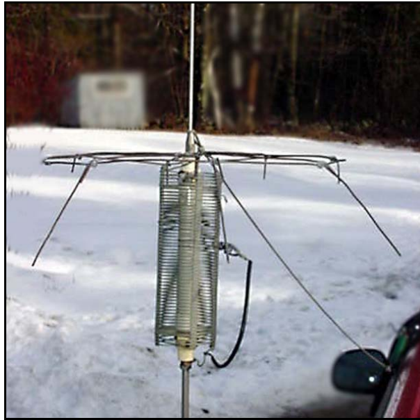
The completed antenna, loading coil and capacity Top Hat installed on my truck. W1RXH photos
