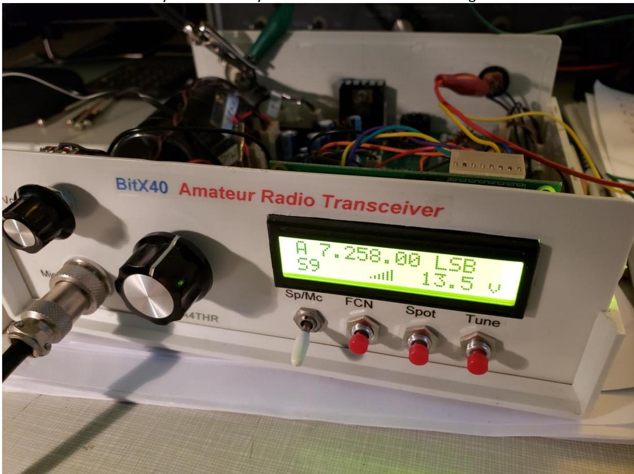
Front panel after adding the power supply voltage
