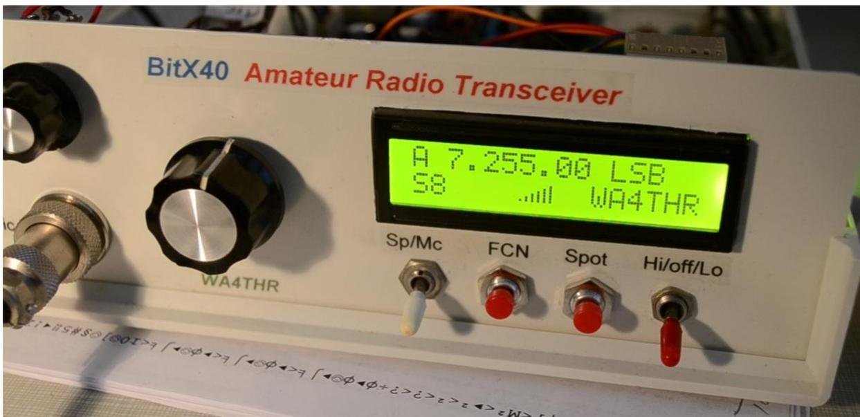
Appearance testing a modification to provide an S-meter
