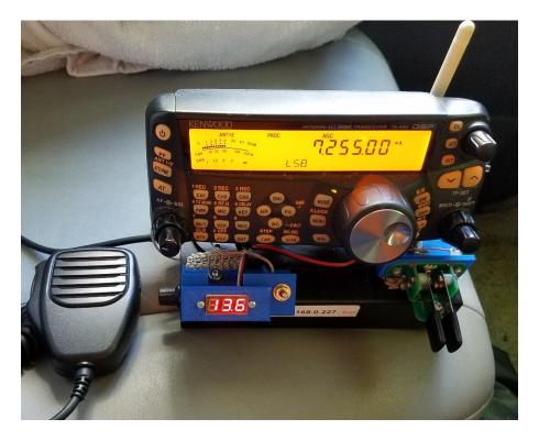
I mounted the control head on the Remoterig box along with paddles and a digital voltmeter. This package can operate using 12 V from the camper or a small rechargeable battery out on a picnic table or in a tent.
