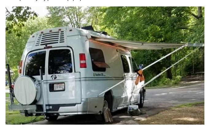
My original plan was to operate a rig inside the van. To that end, I installed a nice Tarheel screwdriver antenna seen in the photo above at the left of the spare tire again with the plan to avoid any setup time needed to put up a wire antenna. As expected it tunes nicely from inside and should be reasonably efficient as a mobile antenna. But things don't always go as expected.
